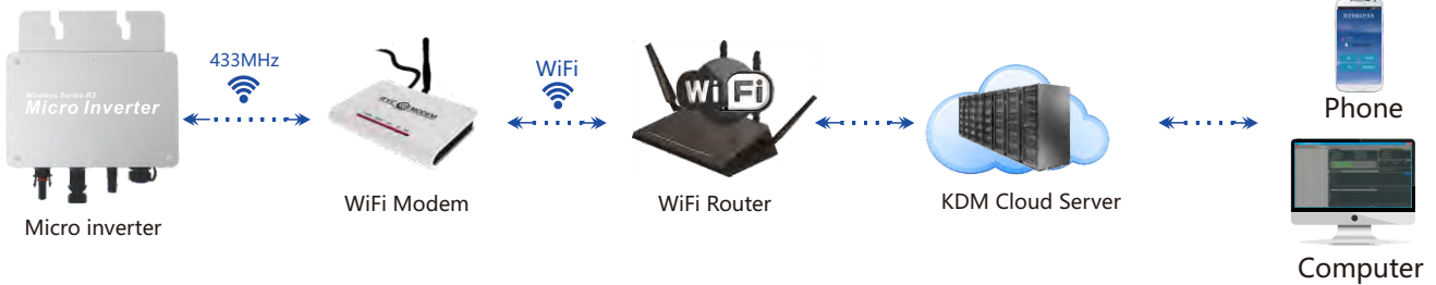
Power monitoring system diagram
